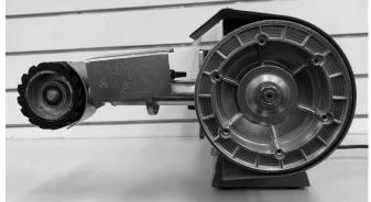
Install the guard (F) over the assembly and tighten the 3 x 6mm cap screws (G)
